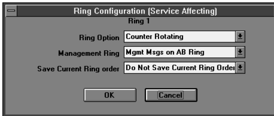
Figure 2-10. Ring Configuration (Service Affecting)
