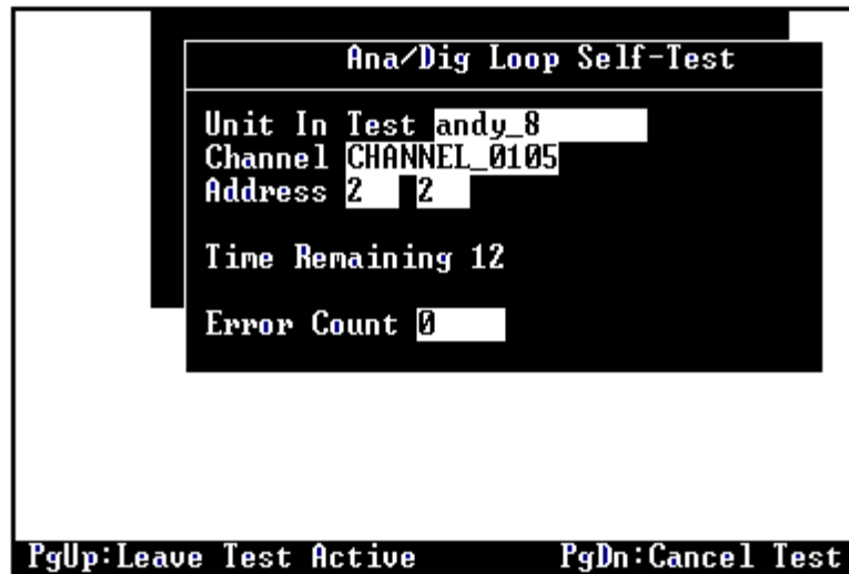
Figure 7-3. ALM Test Status Screen
