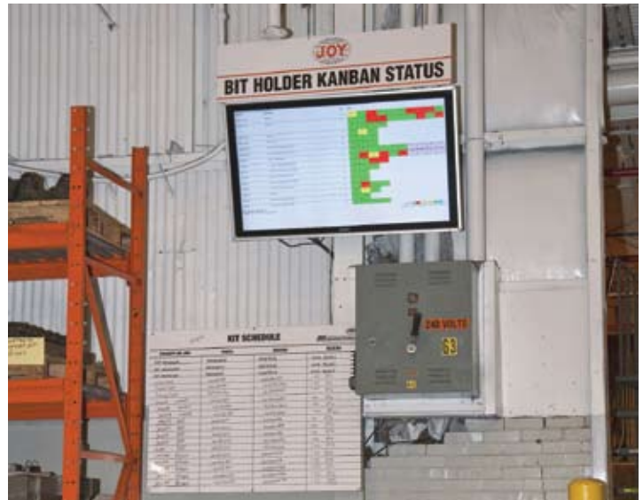
Digital screens are also used to display "Kanban" inventory information in real time. These screens inform workers of which parts are in inventory, which are in transit, and in what bins particular parts are found.
